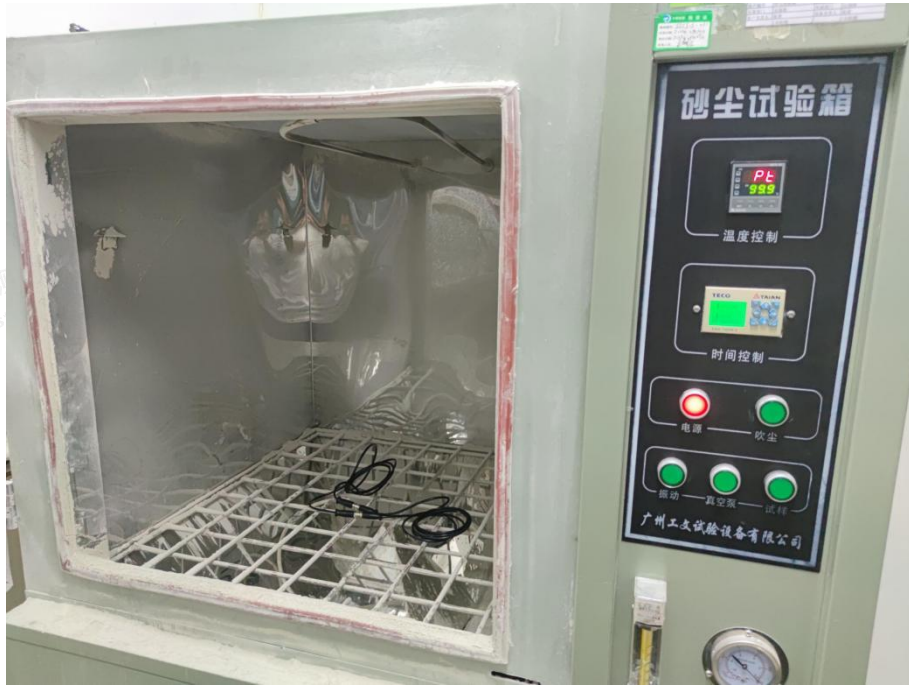
Photo 3: IP6X test of model M12 4 pin
