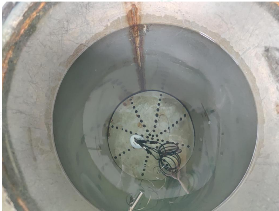
Photo 4: IPX8 test of model M12 4 pin
