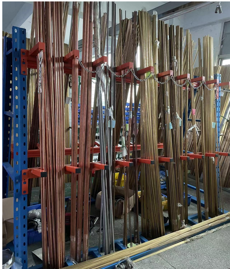
The raw material of connector contacts is Phosphorus bronze from Boway
