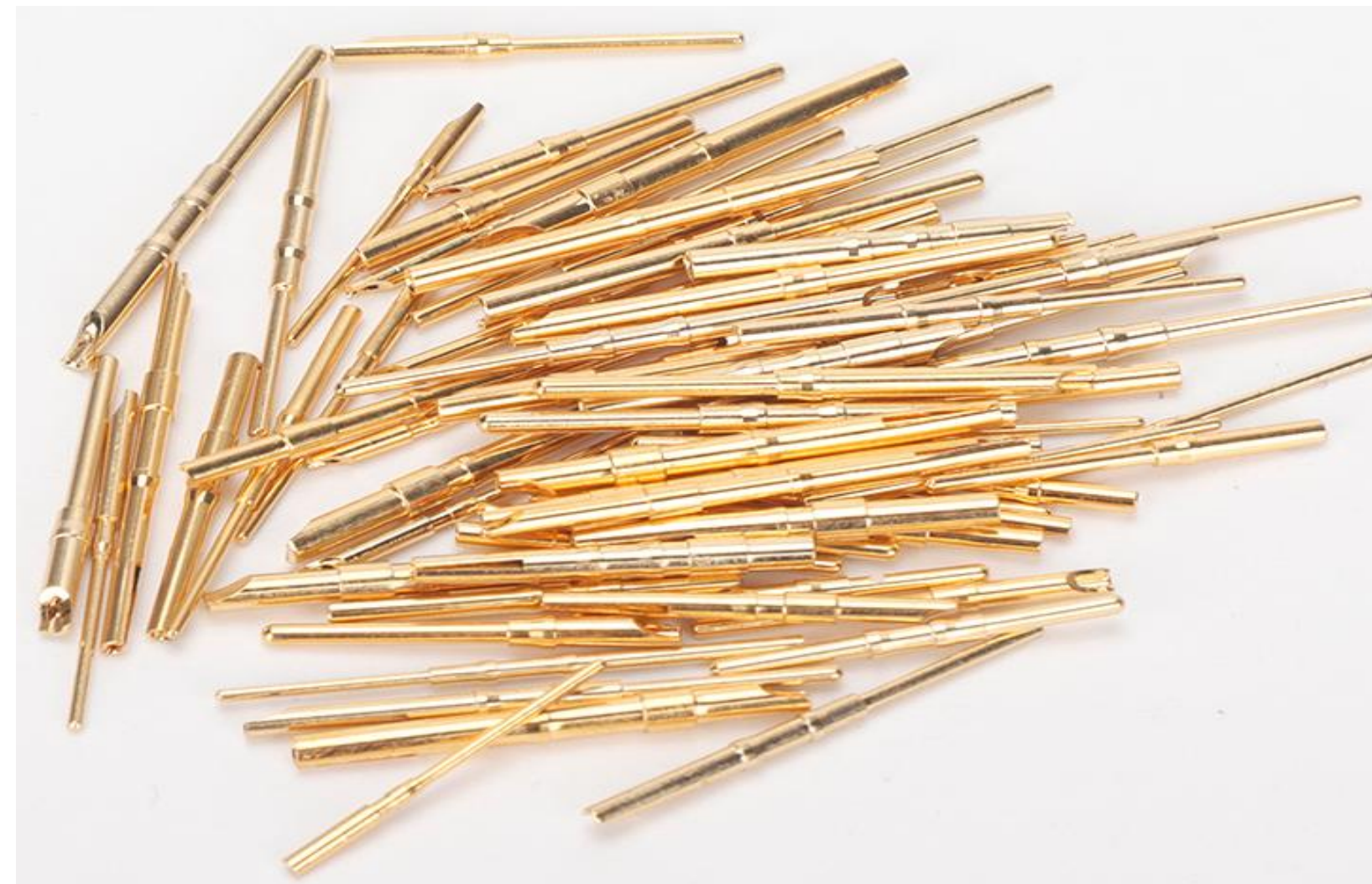
Connector contacts is Phosphorus bronze with 3μ gold plated
