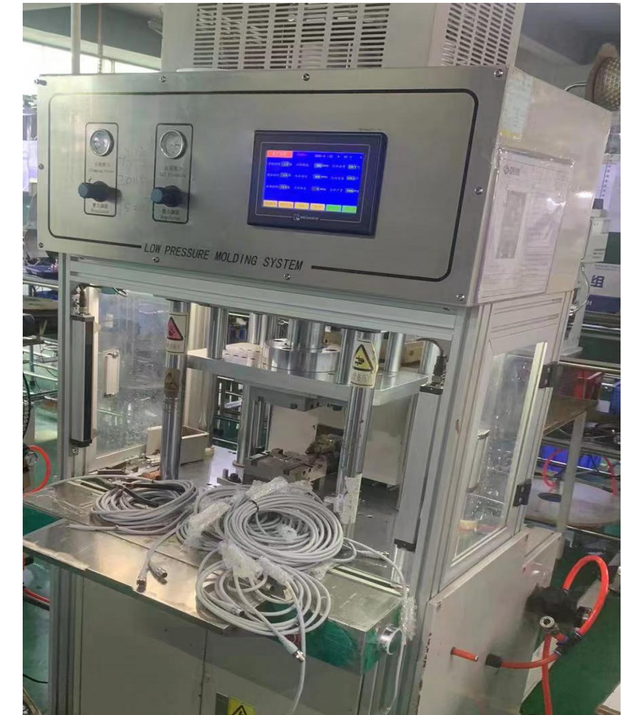
Low pressure injection molding, better waterproof effect
